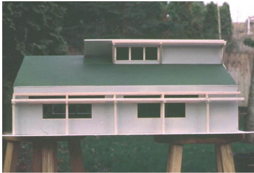
Fig. 21: Daylighting study model
