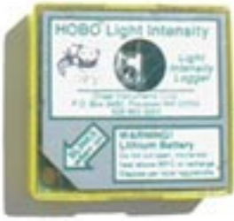
Fig. 43. HOBO light intensity data logger used in Hobopod.
