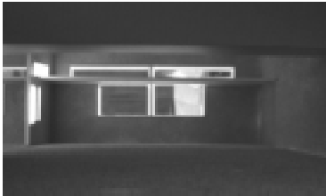
Fig. 31. Solar analysis using a daylight model.
