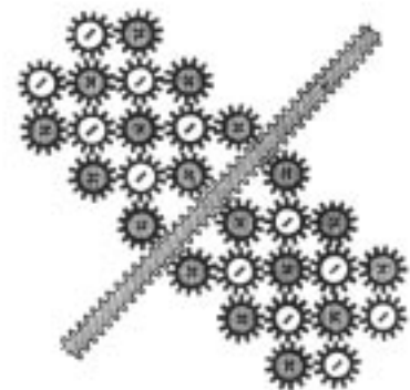
Fig. 1 Lodge's Cogwheel Model of the Ether. The spinning cogwheels represent a magnetic field.
