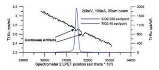
**FIGURE 4.** Wavelength dispersive scans on  $SiO_2$  and  $TiO_2$  at the position for the  $TiK\alpha$  peak showing "holes" in the continuum both adjacent to and directly underneath the analytical peak position. This scan was performed on a LPET analyzing crystal on a Cameca SX-100 EPMA instrument. Similar effects are not always observed on PET, PETJ, or PETH analyzing crystals, which may be due to different mounting orientations of the non-isometric (tetragonal) PET crystal.
