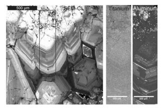
**FIGURE 1.** CL image and Al and Ti trace element WDS maps of vein quartz from the El Salvador porphyry copper deposit, Chile (cf. Rusk et al. 2008), using a JEOL 8900 EPMA. CL image shows early mosaic quartz crystals overgrown by quartz with euhedral growth zones of oscillating CL intensity. CL intensity correlation with Ti concentration is difficult to determine in a  $TiK\alpha$  X-ray map without a proper quantitative background correction.
