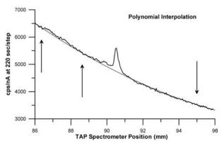
**FIGURE 3.** Wavelength intensity scan data on hydrothermal quartz in the range of the Al $K\alpha$  peak position (black lines). The gray lines represent different background models: linear (top) and polynomial (bottom). The arrows indicate the selected fit positions for the polynomial fit regression model. The choice of background model significantly affects the apparent Al abundance.
