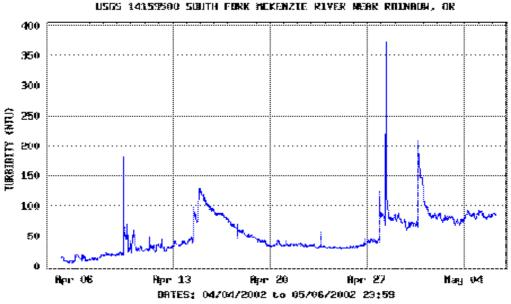
Figure 6: Increases in turbidity as a result of construction at Cougar Dam
