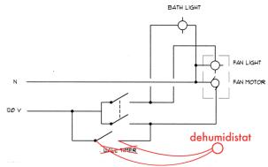
Fig 7: Wiring diagram with dehumidistat
