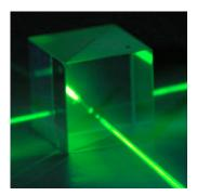
16. More precisely, a beamsplitter contains two input ports and two output ports. Thus, consider two classical fields, with the same polarization and same frequency, entering the two input ports of a beamsplitter. Suppose the complex amplitudes of the (classical) fields are  $\alpha_1$  and  $\alpha_2$ . The beamsplitter produces two output fields with the same polarizations and frequencies, but with different amplitudes:
